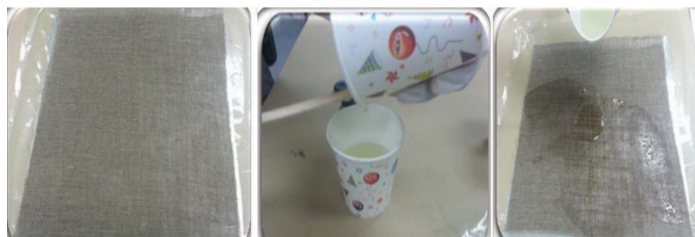
Figure 2. Specimen preparation for epoxy mixture.
