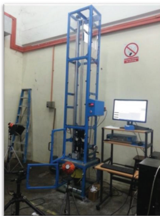
Figure 4. Plate secured in place using the test rig for impact.
