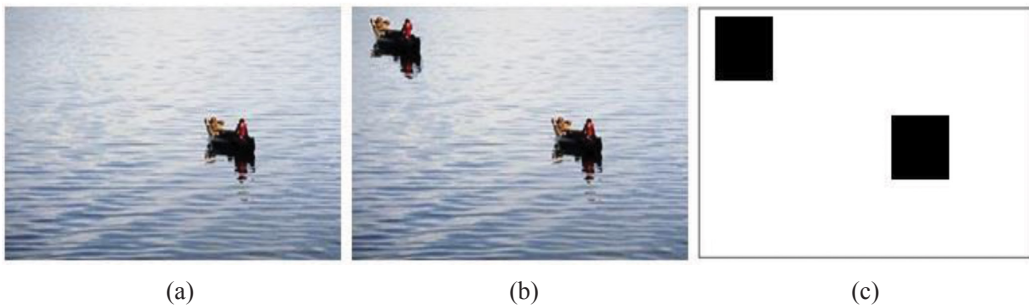
Figure 5. (a) Original image; (b) Forged image; and (c) Detected region of copy-move forgery
