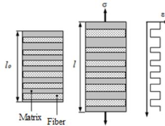
Figure 9. Tensile test perpendicular to fibre position
