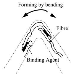
Figure 13. Composite flexibility through fibre flexibility (Arya, 2005)
