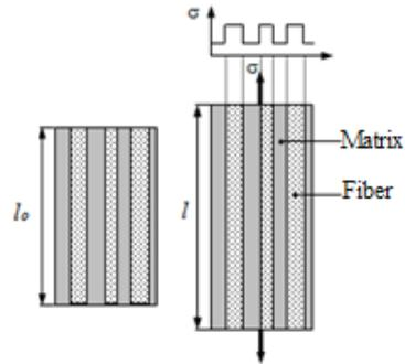
Figure 8. Tensile test parallel to the fibre position
