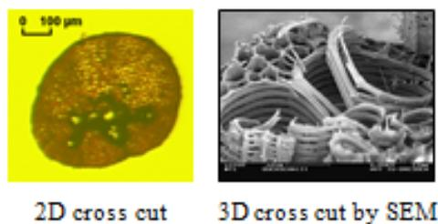
Figure 1. Structure of EFB fibre (Arya, 2005; Arya, 2015)
