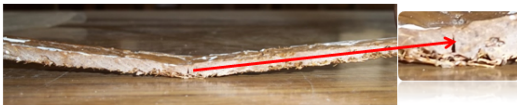
Figure 7. Matrix crack observed in composite specimen
