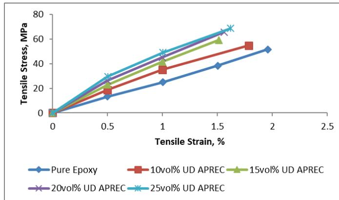
Figure 4. Typical tensile stress-strain curve for Pure Epoxy, 10vol% UD APREC, 15vol% UD APREC, 20vol% UD APREC, and 25vol% UD APREC
