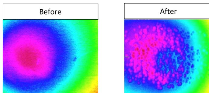
Figure 3. The impacted zones of spot welded joint
