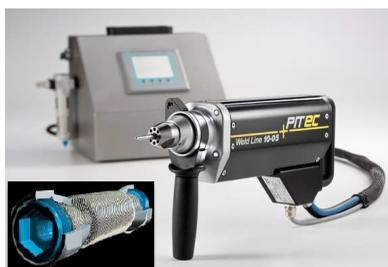
Figure 2. The PIT controller and handheld device (Mohamed, Manurung, Shah, & Othman (2015))
