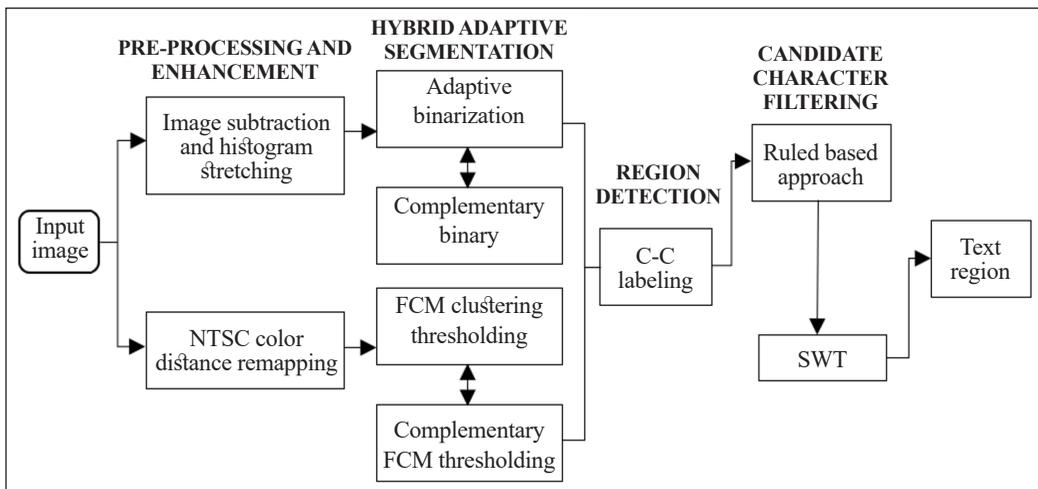
Figure 1. Block diagram of the proposed approach
