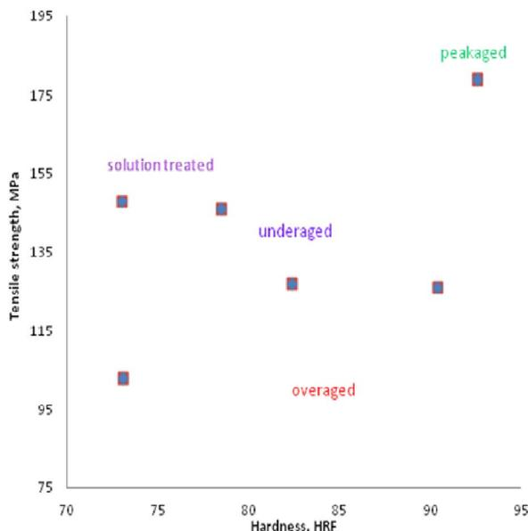
Fig. 2 Ultimate tensile strength as a function of ageing hardness of Al-6Si-0.5Mg-2Ni alloy.
