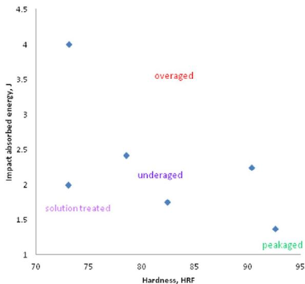
Fig. 5 Impact strength as a function of Rockwell hardness of the Al-6Si-0.5Mg-2Ni alloy in the solution treated, underaged, peakaged and over aged conditions.
