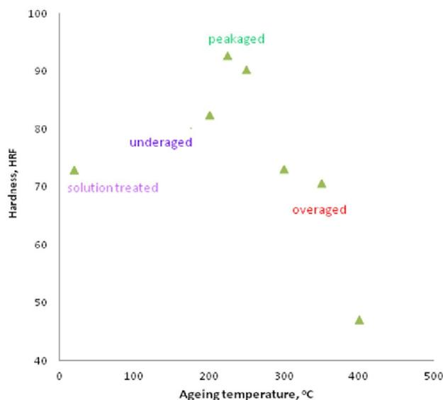
Fig. 1 Variation of hardness of Al-6Si-0.5Mg-2Ni alloy at different ageing temperatures.
