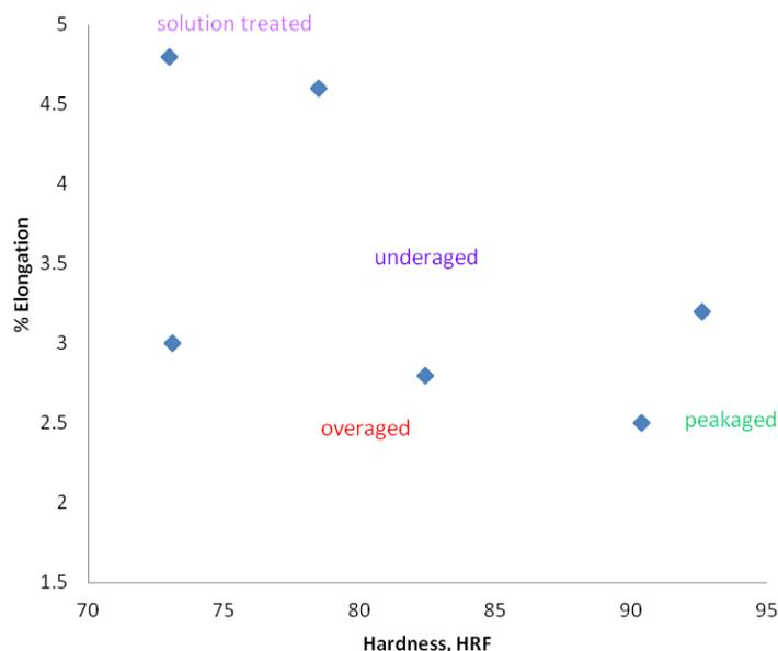
Fig. 4 Ductility as a function of thermal ageing hardness of the Al-6Si-0.5Mg-2Ni alloy.
