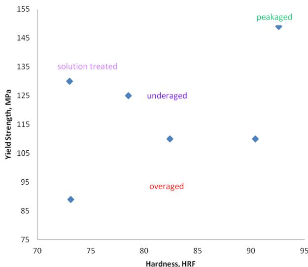
Fig. 3 Yield strength as a function of thermal ageing hardness of the Al-6Si-0.5Mg-2Ni alloy.
