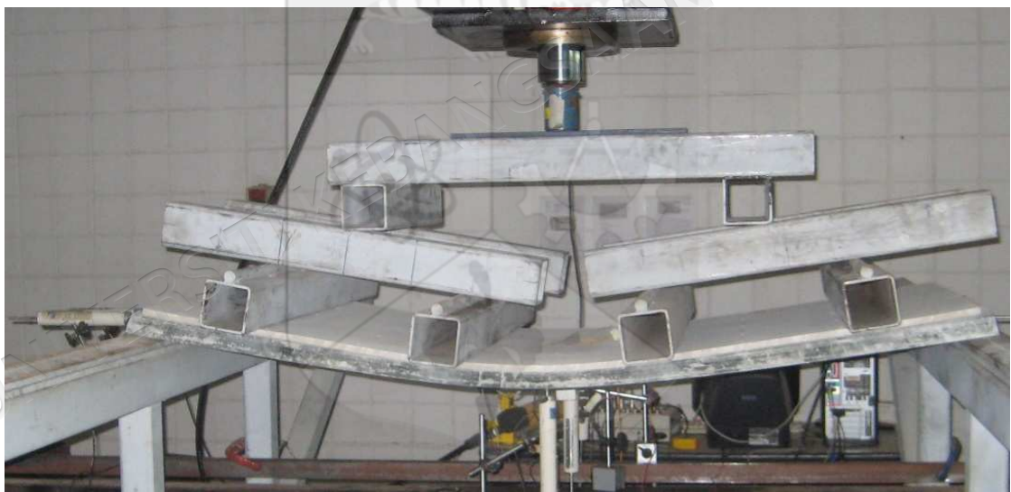
Figure 5.16 Overall buckling of the specimen with simply supported boundary conditions
