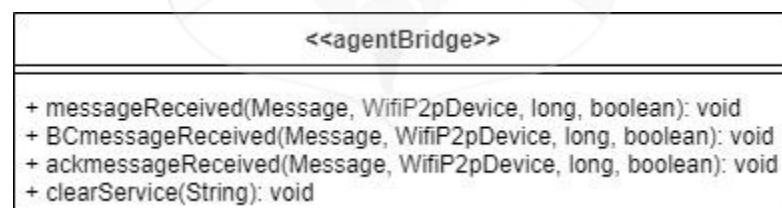
Figure 3.25 agentBridge interface for the implementing class to revert data back to Agent object
