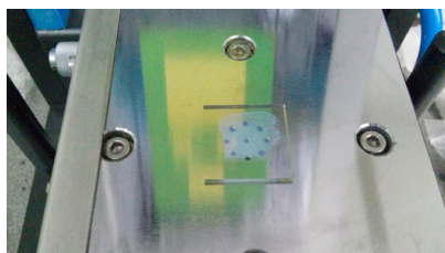
Figure 2. TiO_2 spilled while depositing using screen printing
