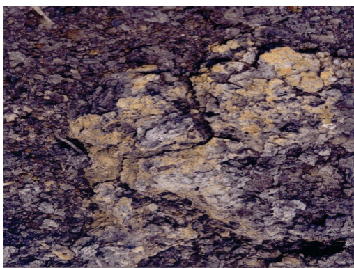
Figure 9. A picture showing yellowish jarosite occurring in the topsoil of the Kelantan Plains Source. Shamshuddin (2006)
