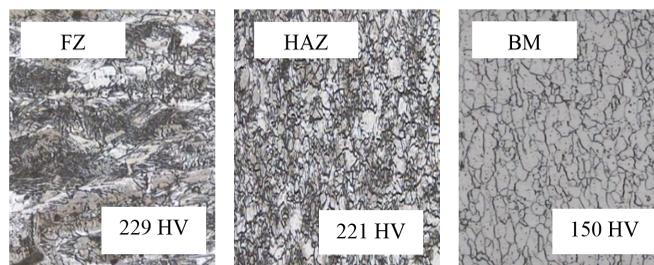
Figure 5. Hardness of the RSW LBIT sample zones
