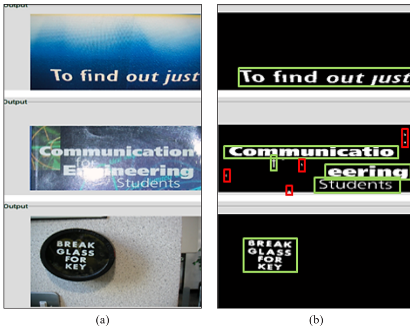
Figure 5. Examples of results of the proposed method for images classified as very complex for extraction: (a) original image set on the left side and (b) text extraction results on the right. (*Red and green line border indicates non-text and text regions subsequently)
