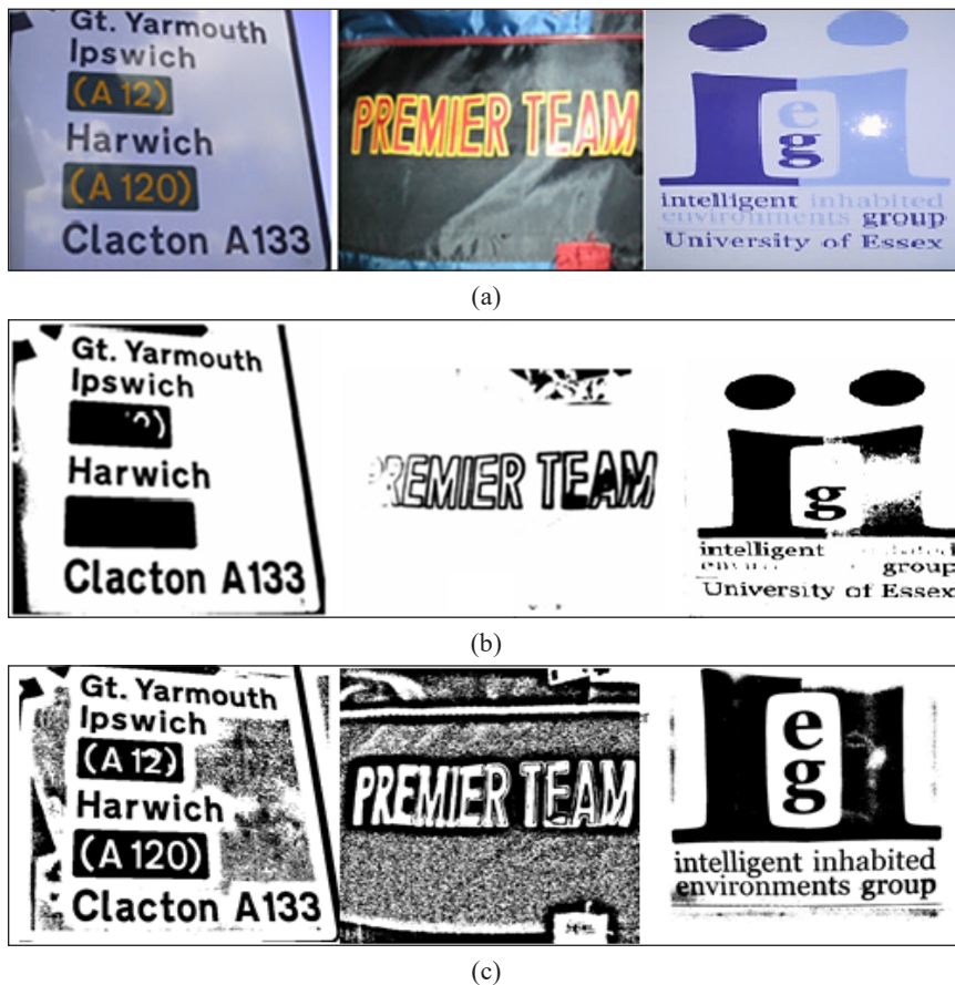
Figure 3. Sample segmentation results. (a) Original image set (b) segmentation results using FCM clustering and (c) segmentation results using adaptive compound binarization.
