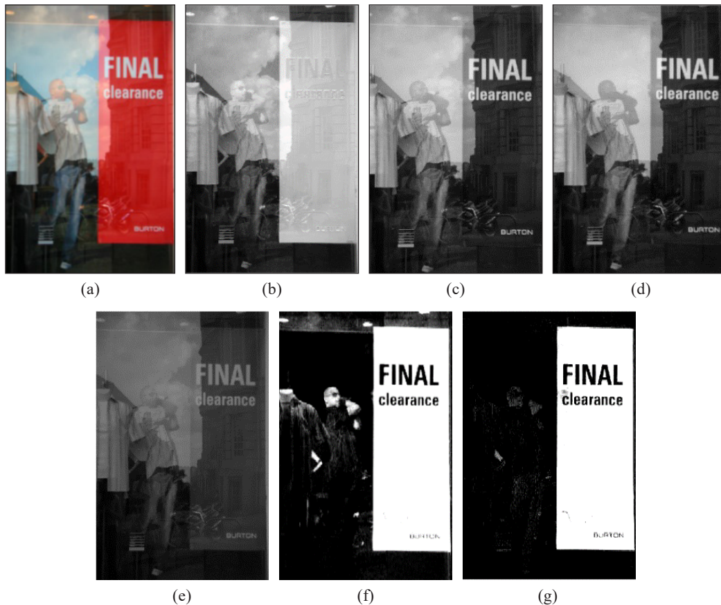
Figure 2. An example showing the effectiveness of the proposed image enhancement method: (a) original image (b-d) before and (e-g) after introduction of the proposed exploited NTSC for image enhancement method according to RGB channels (red, green, blue, respectively).
