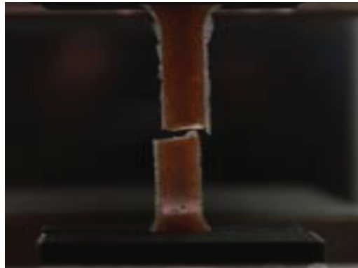
Fig.2: Specimen after tensile test
