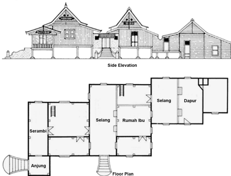
Figure 1. Side elevation and floor plan of a Melaka TMH
