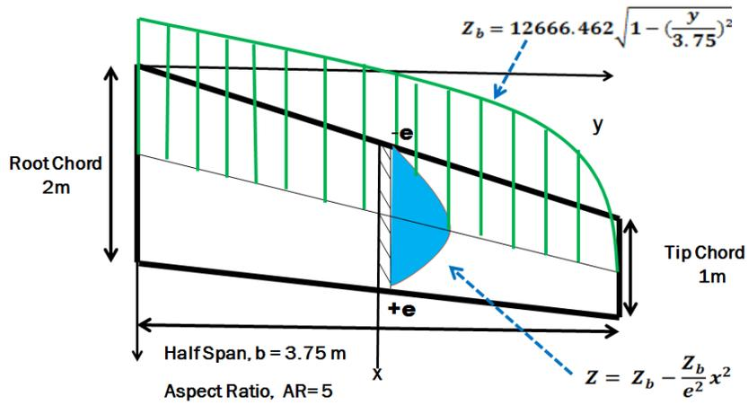
Fig. 3: Wing loading estimation equation.
