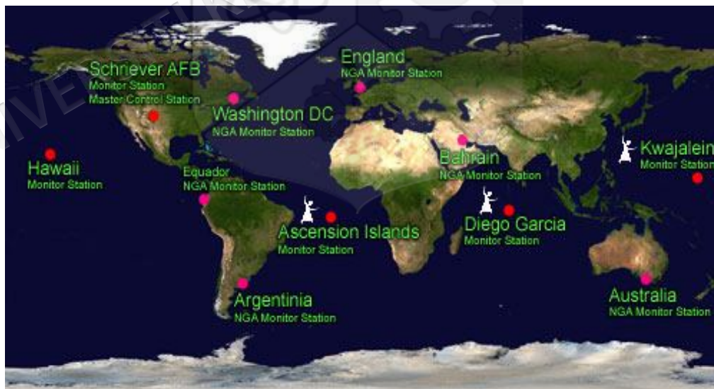
Figure 2.10 The GPS control segment
