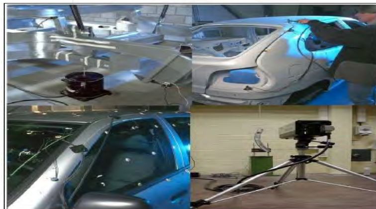
Figure 4.26 Popular excitation and response measurement methods: top left: shaker, top right : impact hammer, bottom left: accelerometers, bottom right: laser vibrometer.
