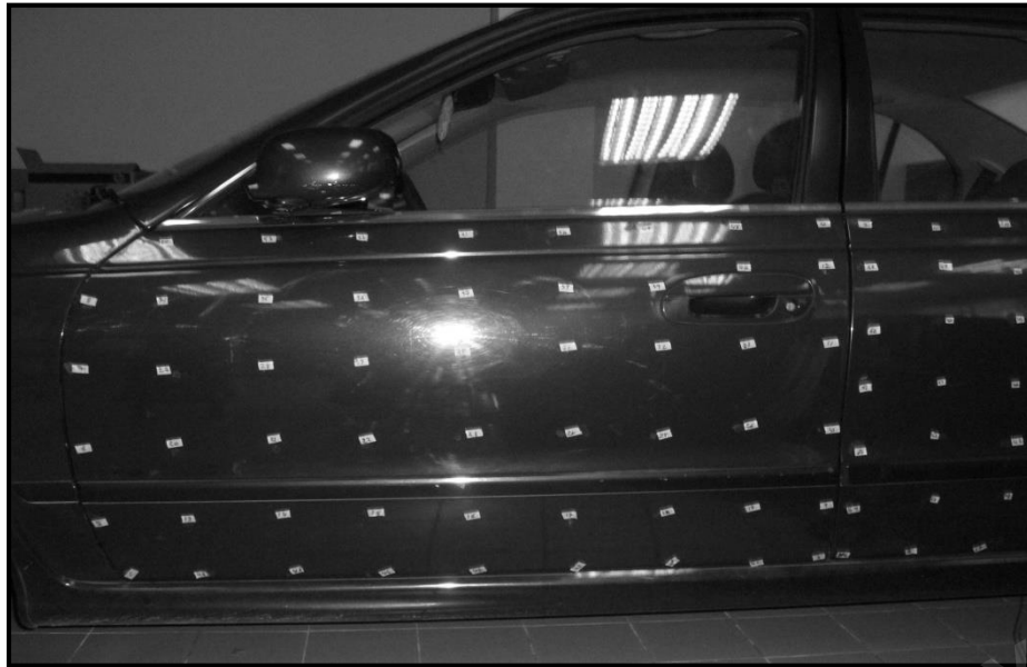
Figure 4.22 Distribution of measurement points over the door panel.
